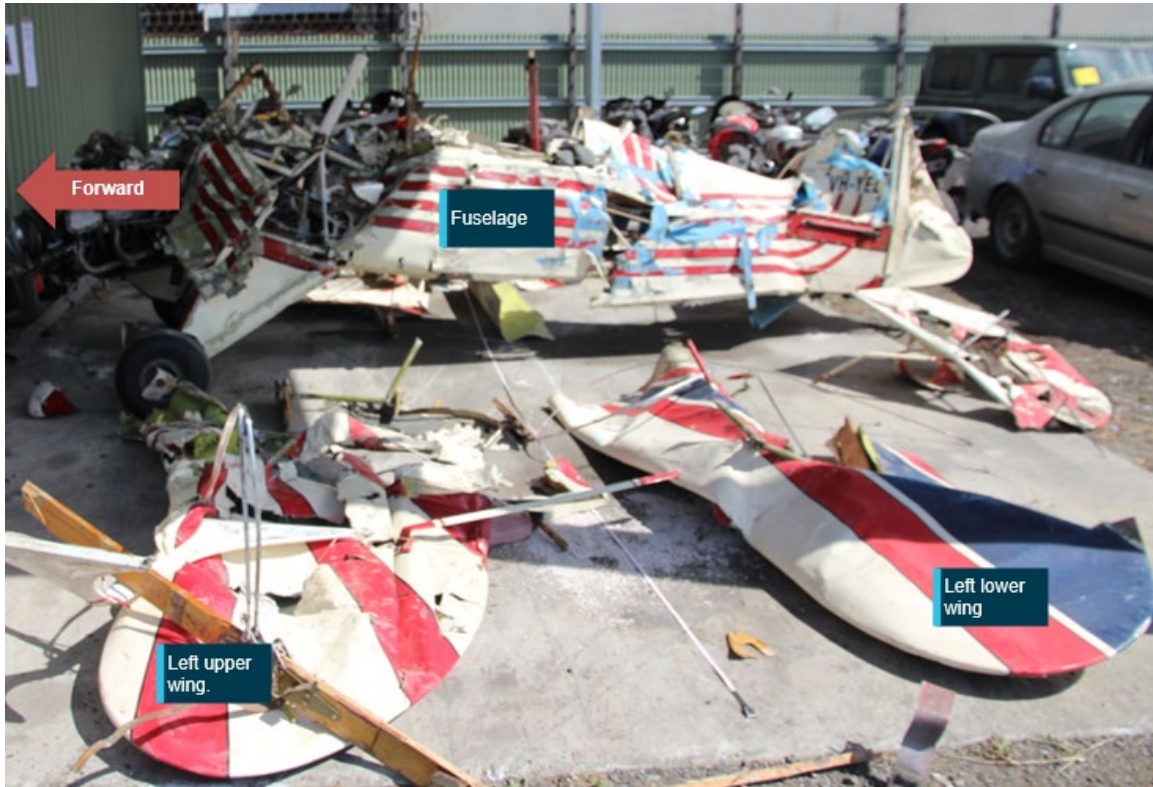
Figure 6: VH-YEL as recovered and partially reassembled
