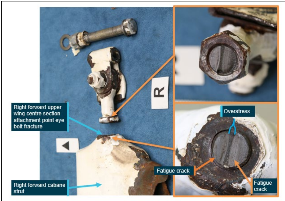
Figure 7: Right eye bolt, cabane strut and fracture surface
