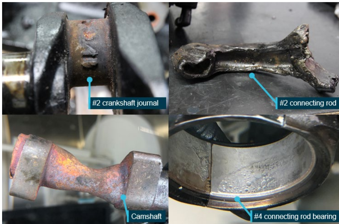
Figure 6: Damaged engine components removed from VH-UQI
