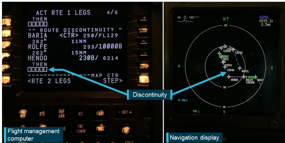
Figure 7: Flight management computer (left) and navigation display (right) showing the discontinuity
