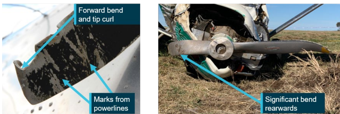
Figure 6: Damage to propeller from powerlines and ground impact
