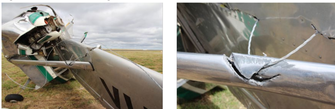
Figure 5: Powerline, left wing and strut
