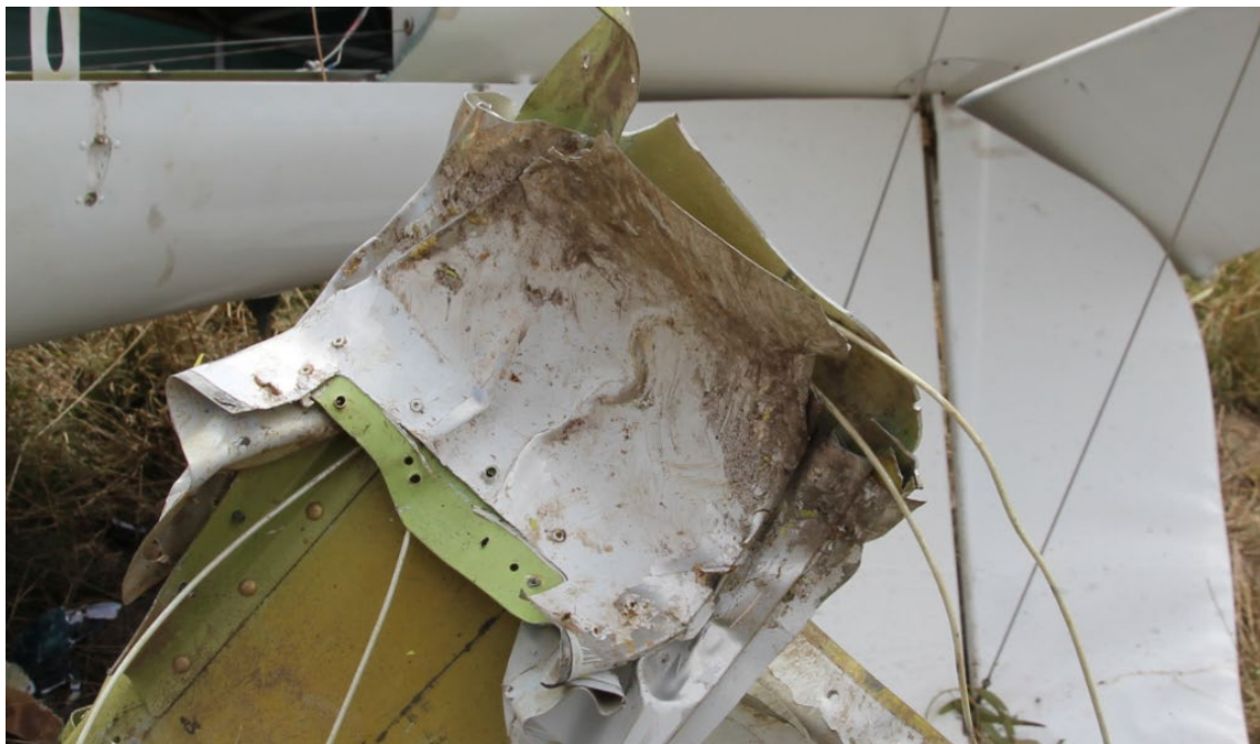
Figure 6: Outboard section of left wing with tree impact damage
