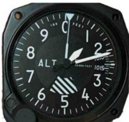
*This altimeter shows an altitude of 1,210 ft (10,000 ft pointer indicating 0, 1,000 ft pointer indication 1,000 ft and 100 ft pointer indicating 210 ft.*
