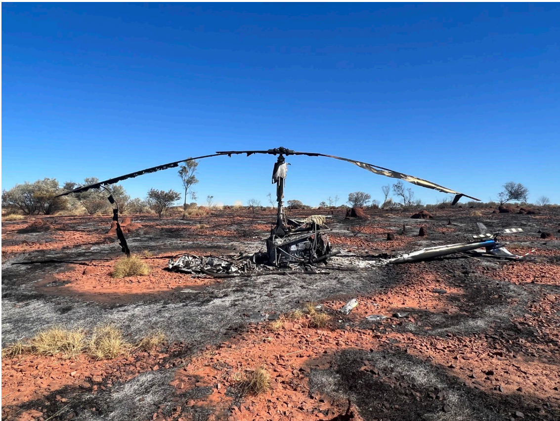
Figure 1: Fire damage to the helicopter and surrounding bushland
