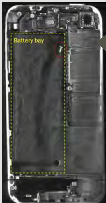
X-ray showing loose screw in the battery compartment
