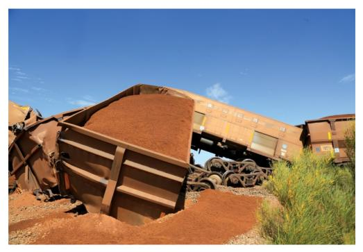
Figure 9: Derailed, loaded iron ore cars located in the rear portion of train M03544
