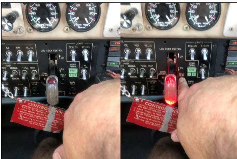
Source: Aircraft maintainer Note: the image is only intended to illustrate the handle warning light. It is not intended to represent the landing gear configuration at the time of the occurrence.
