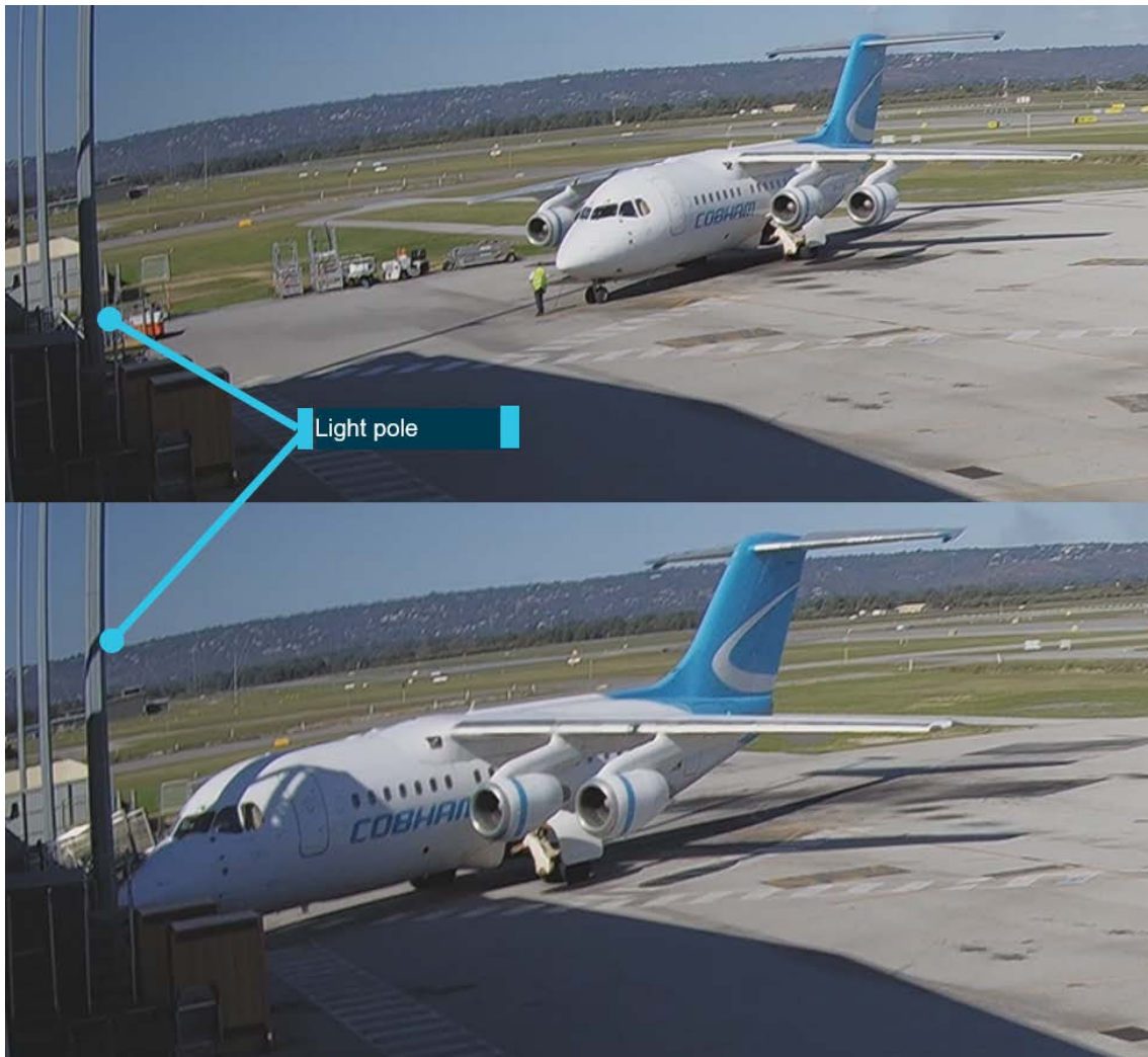
Figure 1: CCTV showing start of roll-forward (top) and collision with infrastructure (bottom)
