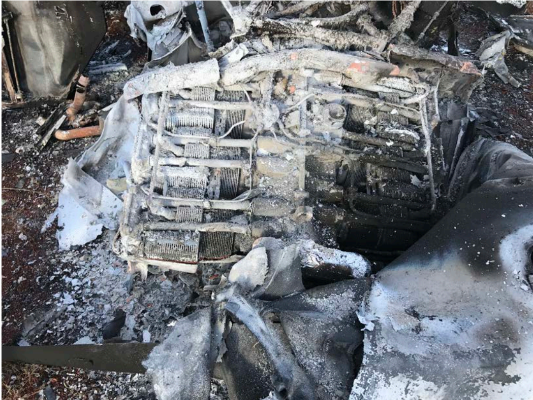
Figure 2: Fire damage to engine
