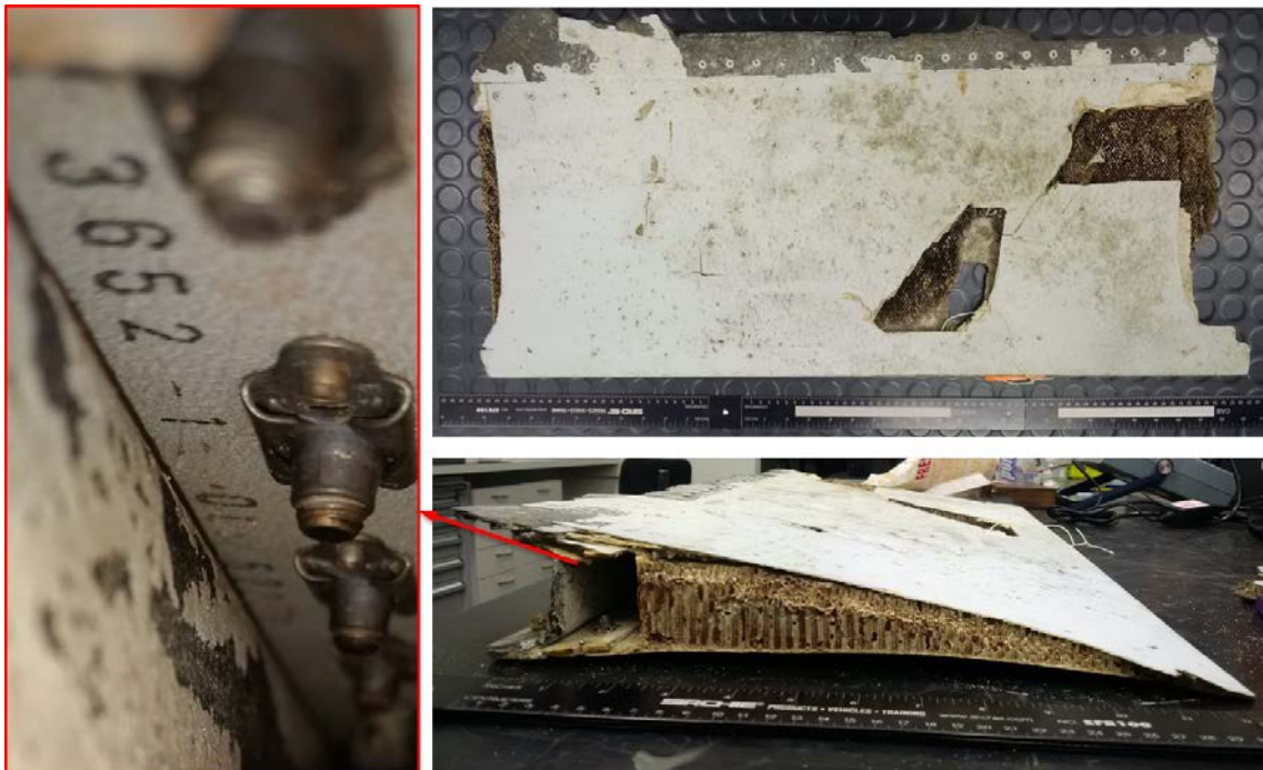
Figure 1: Left outboard flap trailing edge section showing part identification numbers
