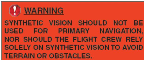
A similar warning was contained in the Primus Apex Smart View supplement to the aircraft flight manual.
