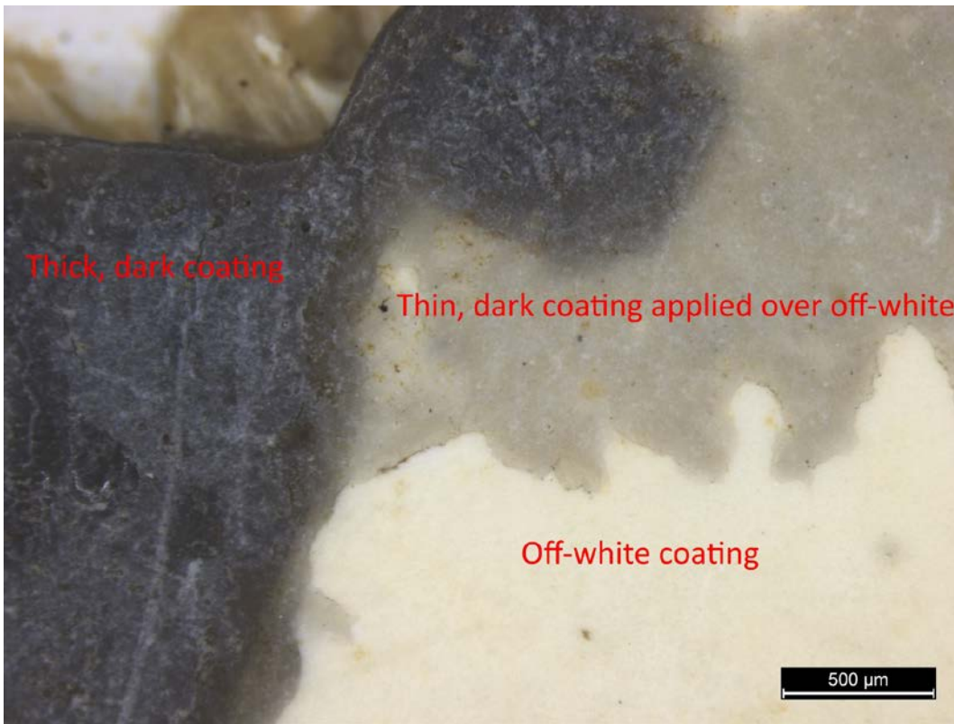
Figure 4: Close-up of applied coatings
