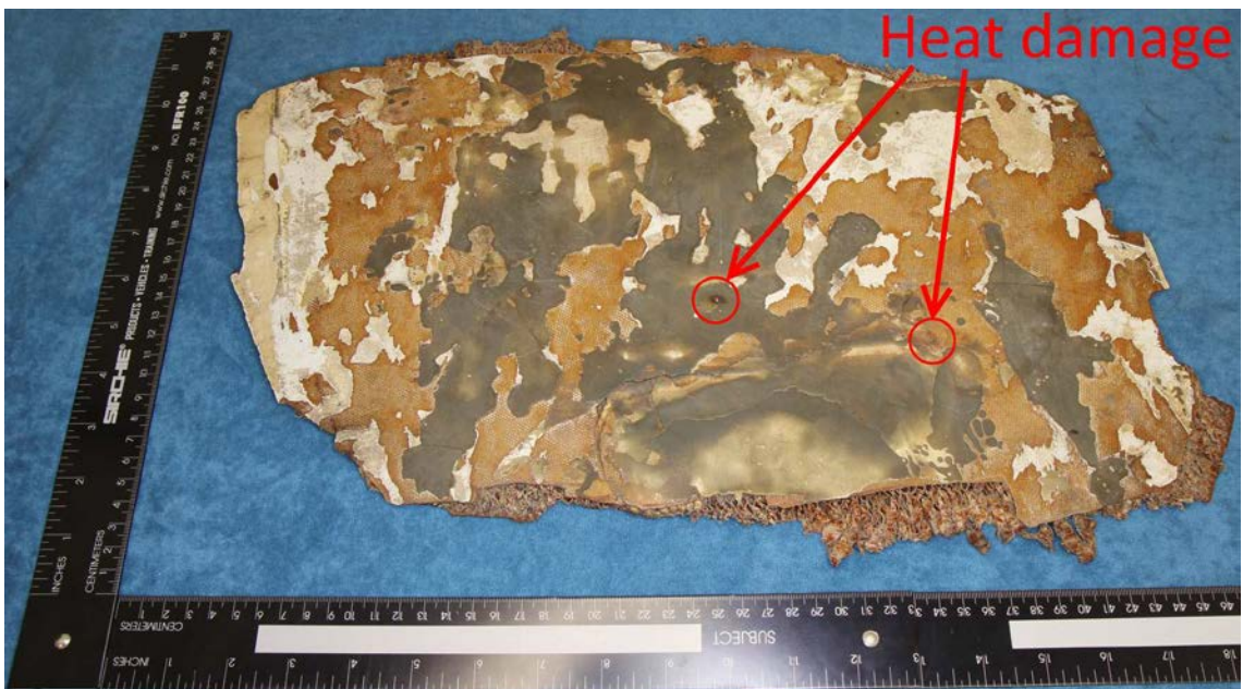
Figure 3: Reverse side of larger composite panel showing discrete areas of heat damage
