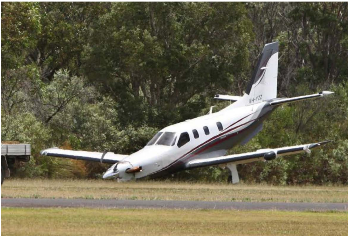
Figure 3: YZZ post-accident showing the damage to the forward section of the aircraft as a result of the nose gear collapse and skidding on the ground
