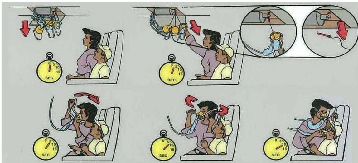
The safety card in your seat pocket gives step-by-step instructions on how to use the oxygen mask. Figure 2 shows an example of an oxygen mask being used by a passenger. Once the oxygen masks drop, grab the one nearest to you, pull it sharply downwards to start the flow of oxygen, fit the mask and secure the strap behind your head.
