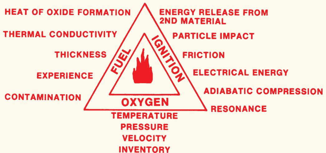
**Figure 17:** The extended fire triangle indicating some of the factors to be considered in a design.
