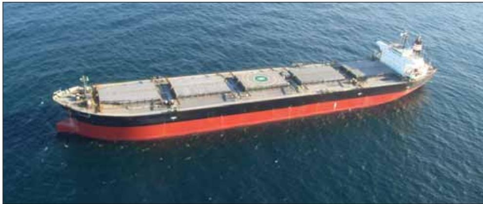
Propulsive power is provided by a five cylinder Mitsui B&W 5S60MC, single acting, direct reversing two-stroke diesel engine developing 10 223 kW. The main engine drives a single fixed pitch propeller which gives the ship a service speed of about 14.5 knots<sup>2</sup>.
