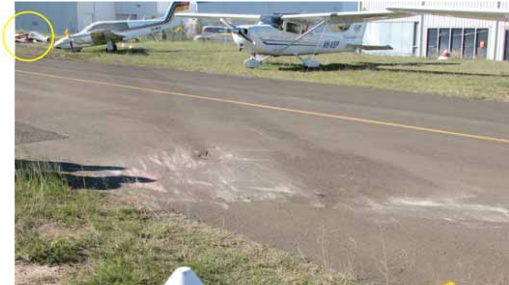
Figure 3: Impact marks on airport taxiway (wreckage circled)
