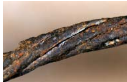
Figure 3 (top left). Illustrates the extent of the corrosion damage to the outer wire strands adjacent to the fracture.
