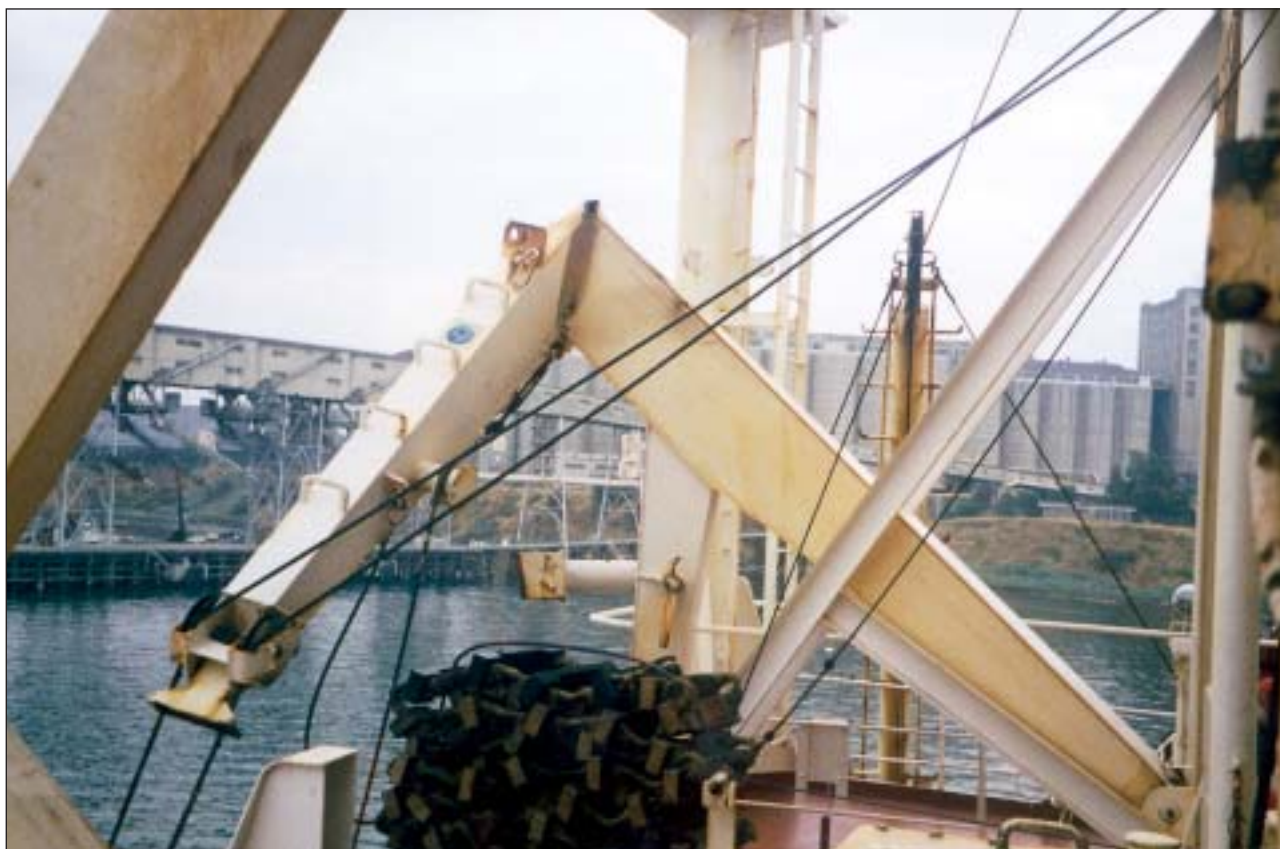
FIGURE 7: Damage to port lifeboat davit
