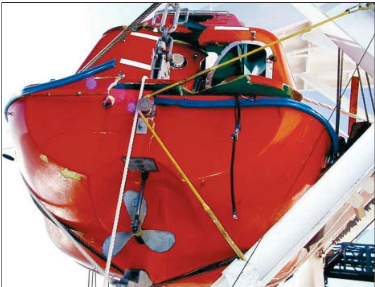
FIGURE 7: Damage to the stern of Washington Trader's port lifeboat
