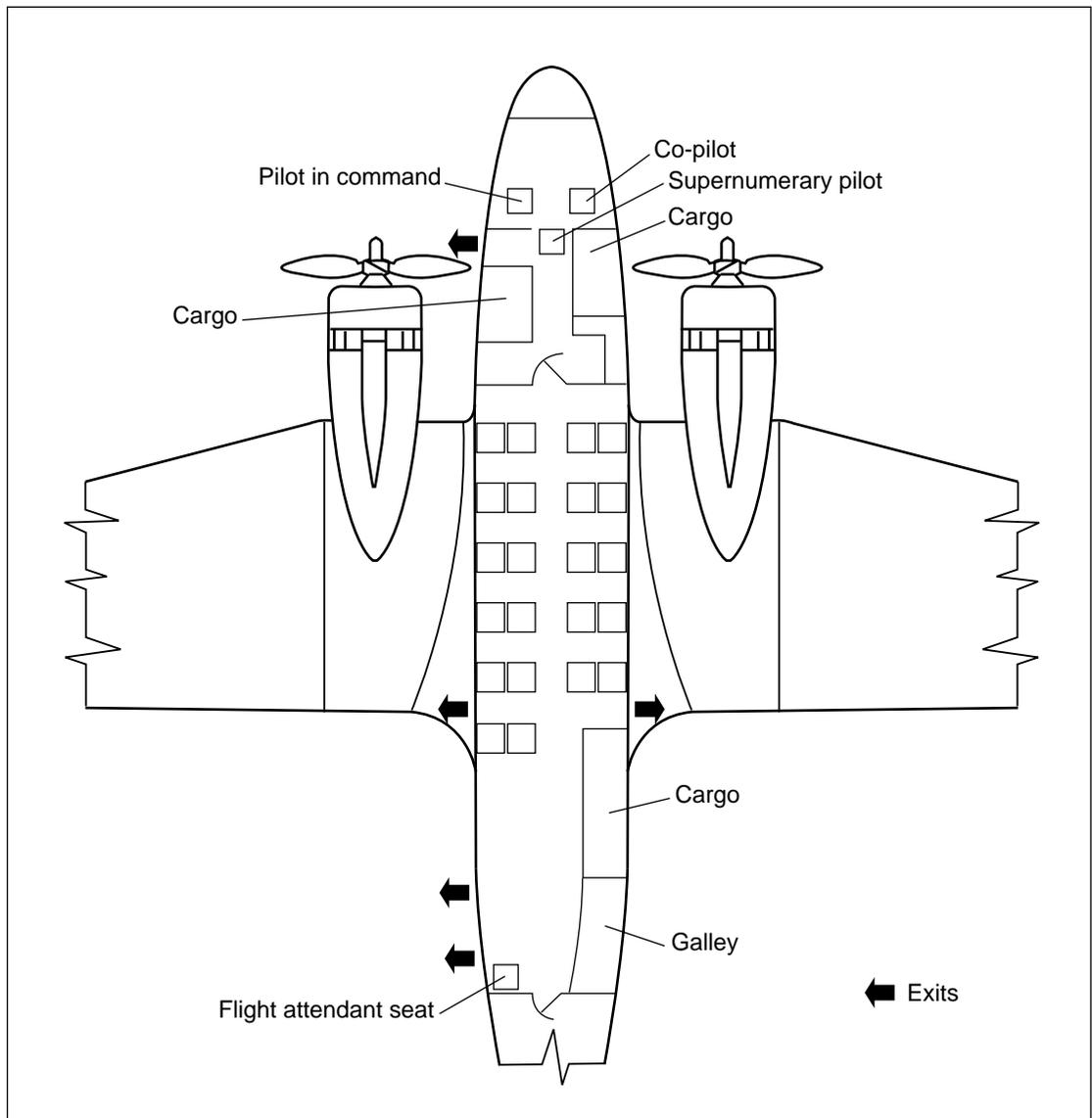
Figure 5. Diagram showing the internal layout of VH-EDC.
