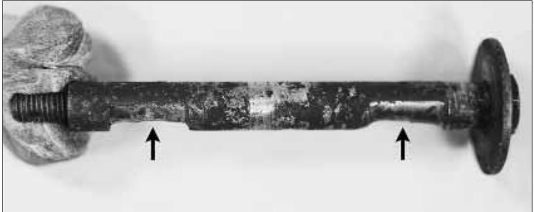
**Figure 4.** The worn pulley block securing bolt.
