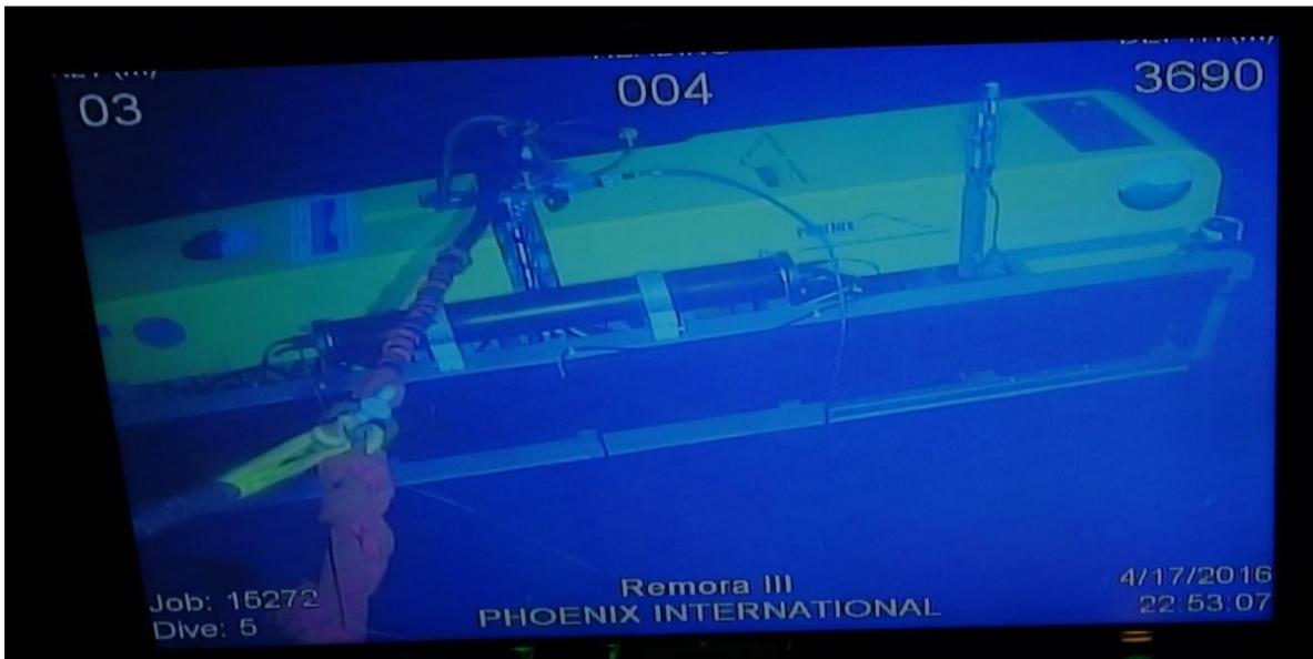
ROV video image of the SL HydroSpheric SLH-ProSAS-60 deep tow system being prepared for lifting to the surface. Source: ATSB, photo by Mel Proudlock
