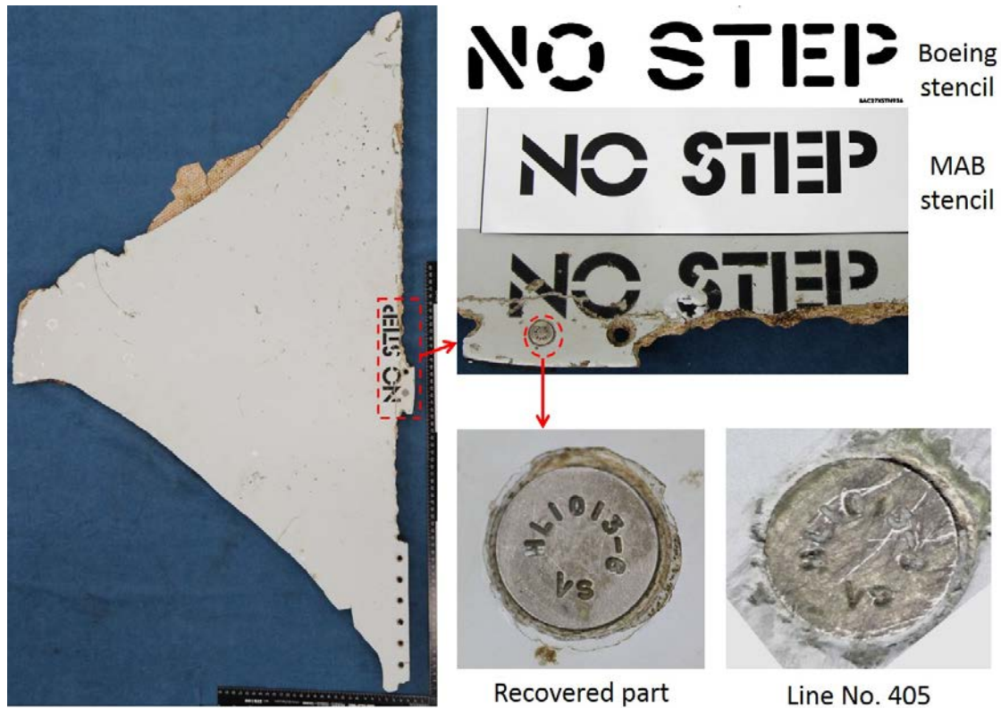
Figure 4: Stabiliser panel “NO STEP” stencil and fastener comparison
