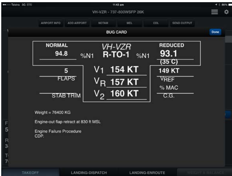
Figure 4: Bug card showing the correct take-off weight (76,400 kg) and speeds
