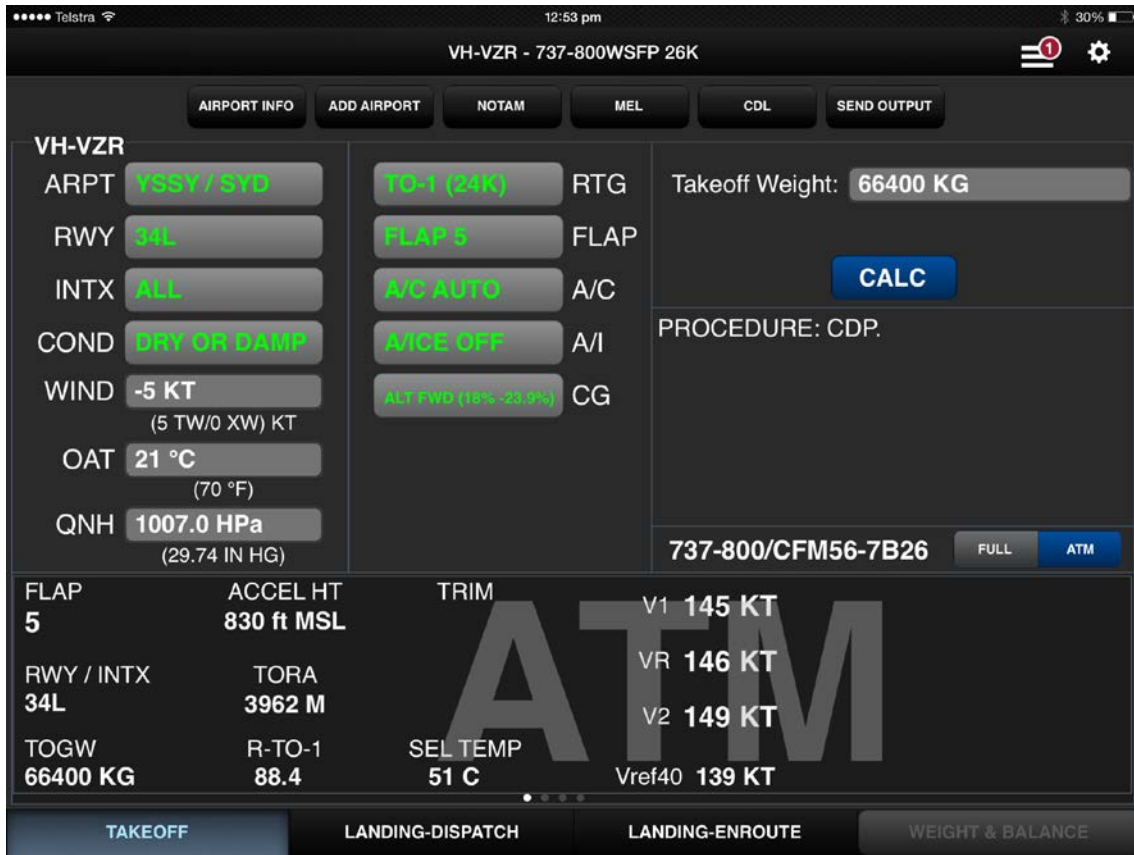
Figure 2: Take-off data entry screen in the on-board performance calculation tool for VH-VZR showing the erroneous take-off weight (66,400 kg)
