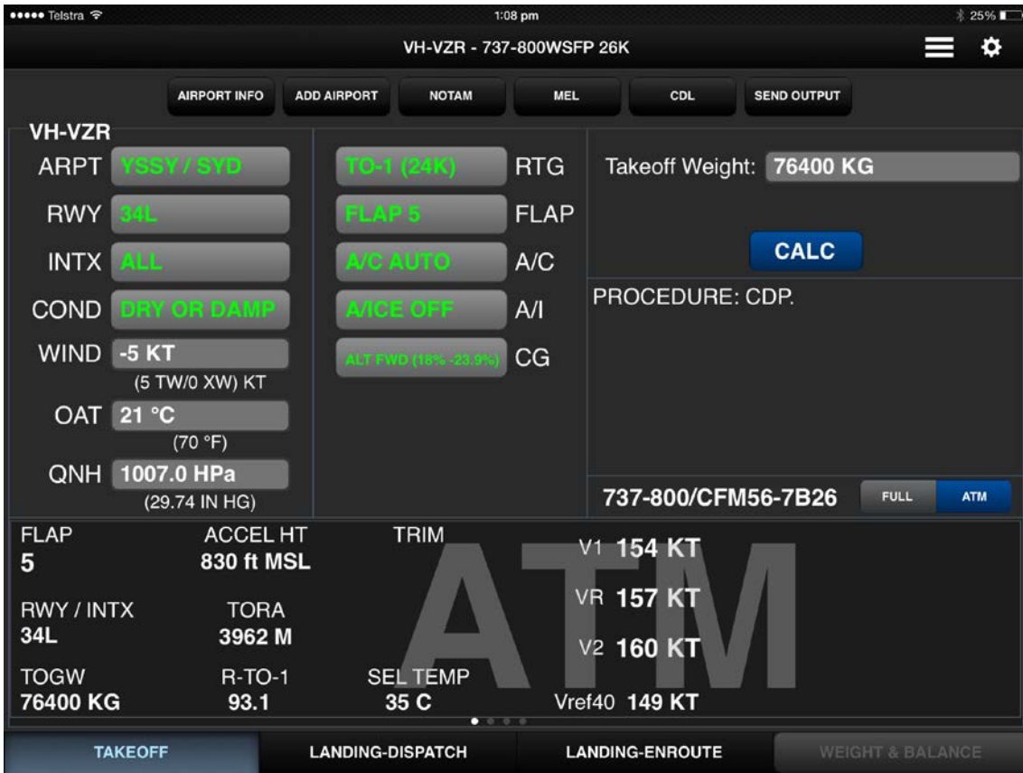
Figure 3: Take-off data entry screen in the on-board performance calculation tool for VH-VZR showing the correct take-off weight (76,400 kg)
