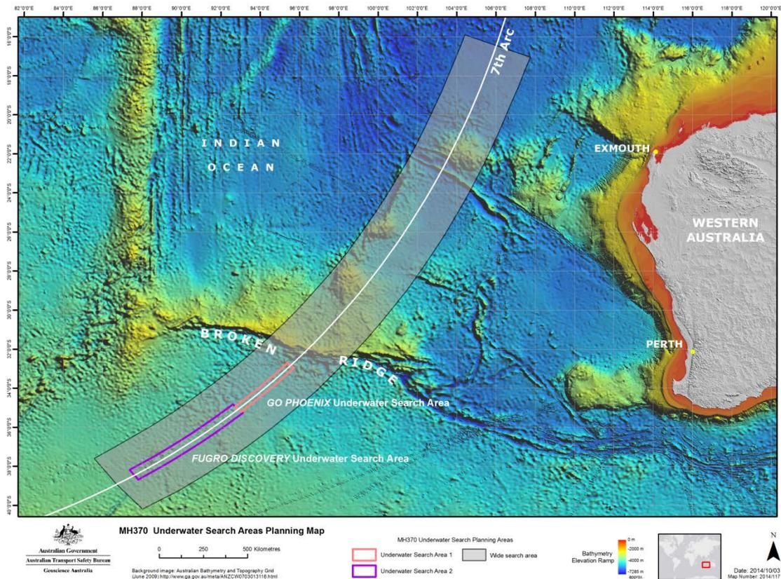
The first area to be searched has been assigned to *GO Phoenix*. It has already been surveyed to ensure an accurate understanding of the sea floor topography. The second area, assigned to the Fugro vessels, is currently in the process of being surveyed.
