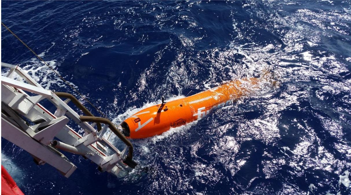
The HUGIN 4500 AUV in the water. Source: ATSB, photo by Fugro.
