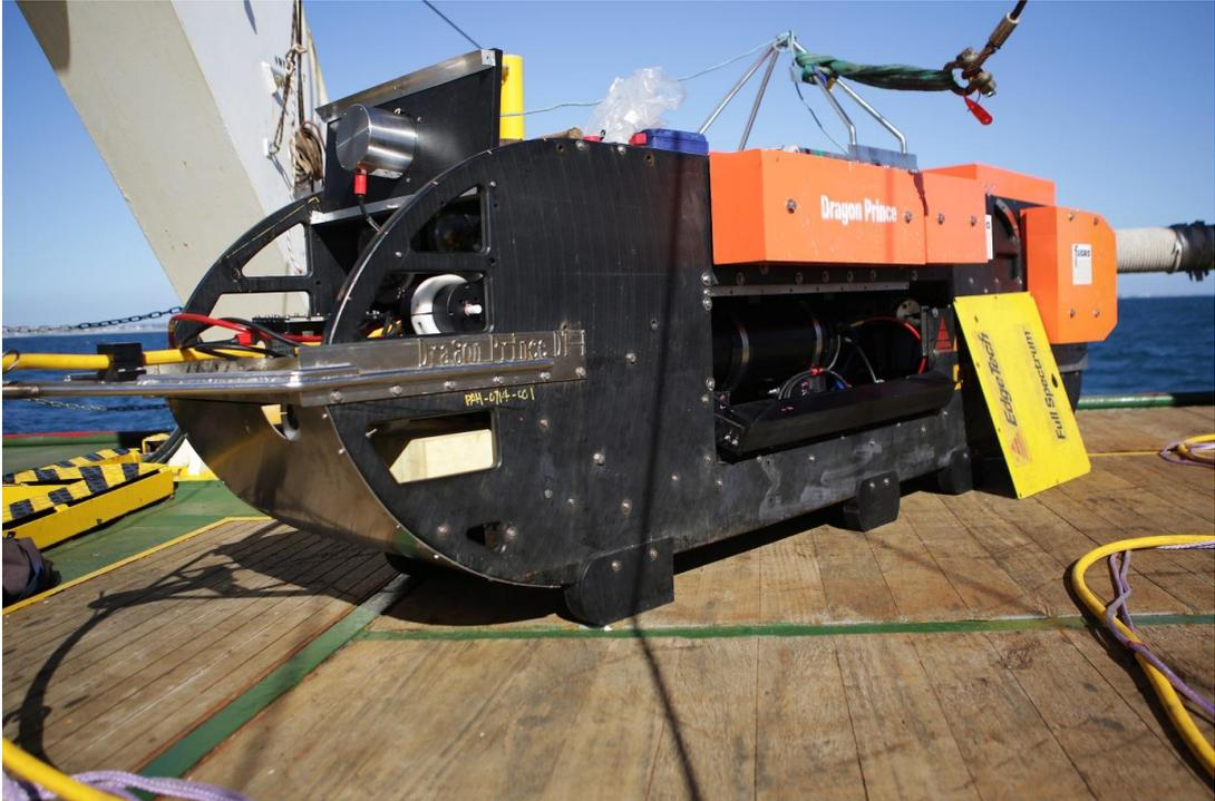
'Dragon Prince', the EdgeTech DT-1 towfish that is being used to search the seafloor for MH370, on the deck of *Fugro Discovery*. Source: ATSB, photo by ABIS Chris Beerens, RAN.
