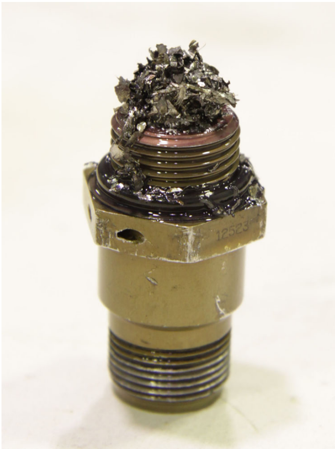
Figure 7: The contaminated magnetic chip detector plug
