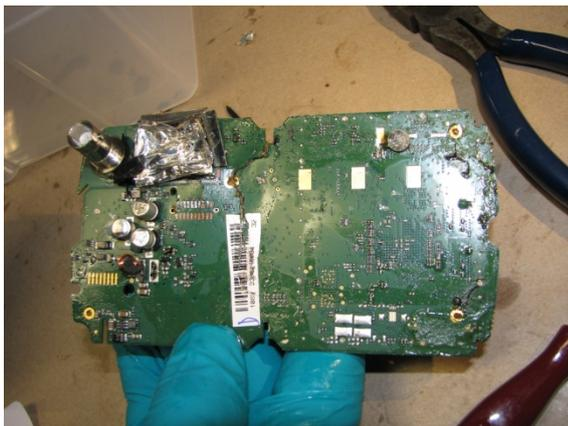
Several electronic devices had become separated from the circuit board. With assistance from the French Bureau d'Enquêtes et d'Analyses (BEA), the French national accident investigation agency, the memory device containing the data was identified.
