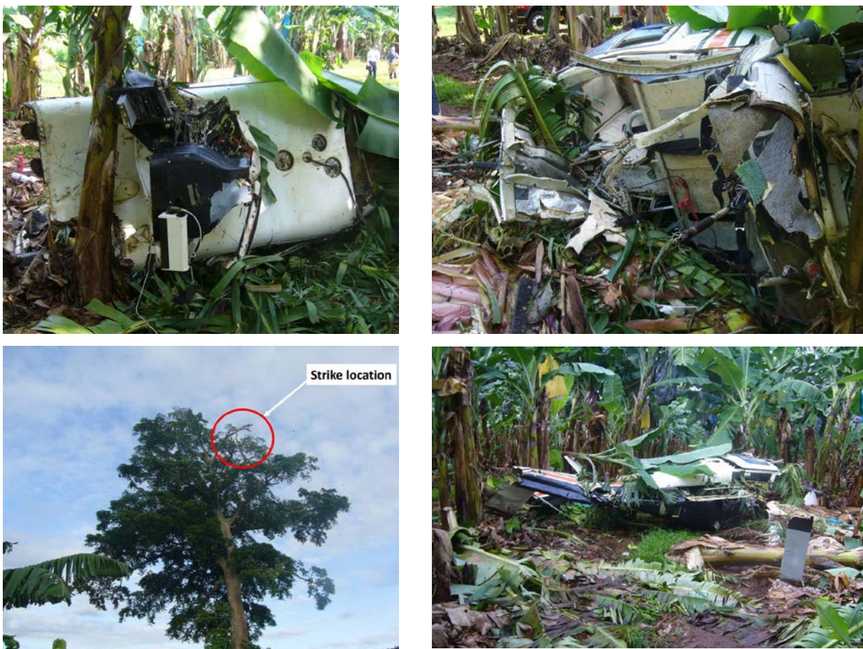
Figure 1: Damage to VH-BNG and large tree strike
