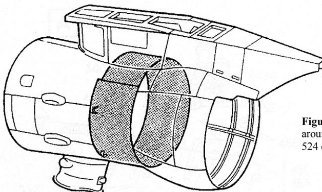
**Figure 2.** Location of the combustion fairings around the gas generator section of the RB211-524 engine core.
