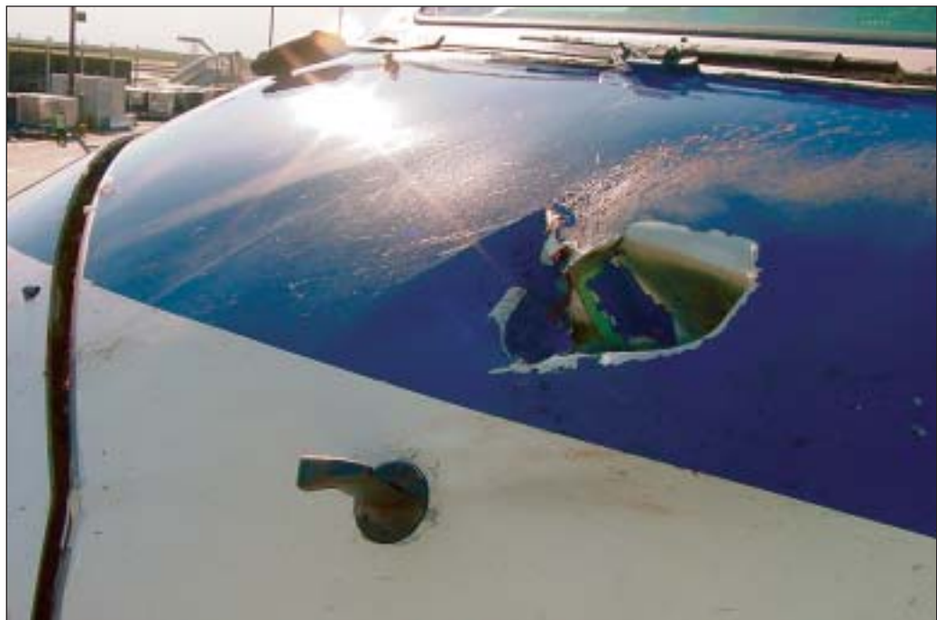
FIGURE 2. Birdstrike damage (B767)
