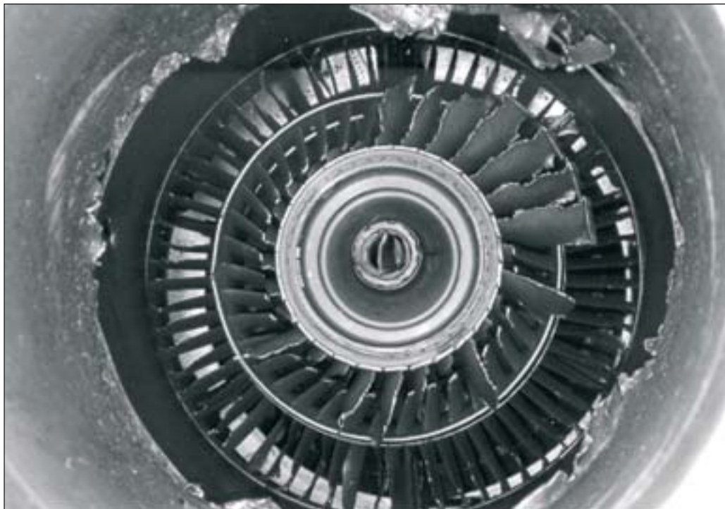
FIGURE 1. Engine damage from bird ingestion
