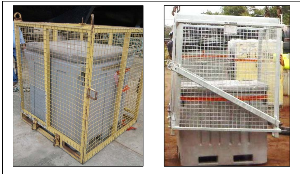
Figure 10: Cage frames now in use for top lifting of containers
