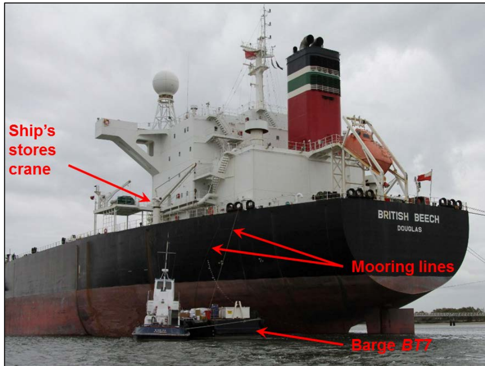
Figure 5: British Beech , tug and barge tie-up arrangement
