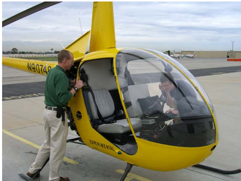
Figure 7.1: The RHC Strain Gauge Instrumented R22
