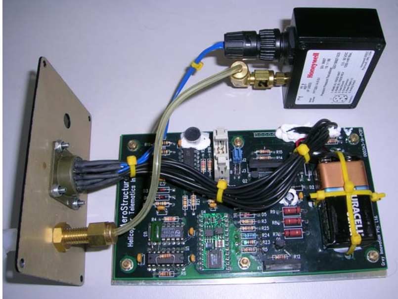
Figure 3.2: Custom Instrumentation Module for the R22 Usage Survey
