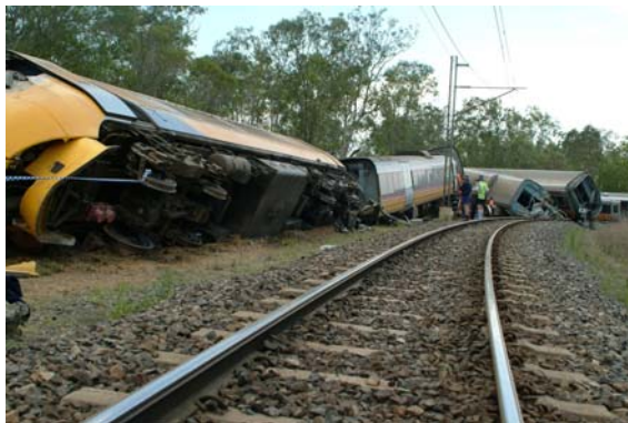
Figure 4: Derailed Cairns tilt Train
