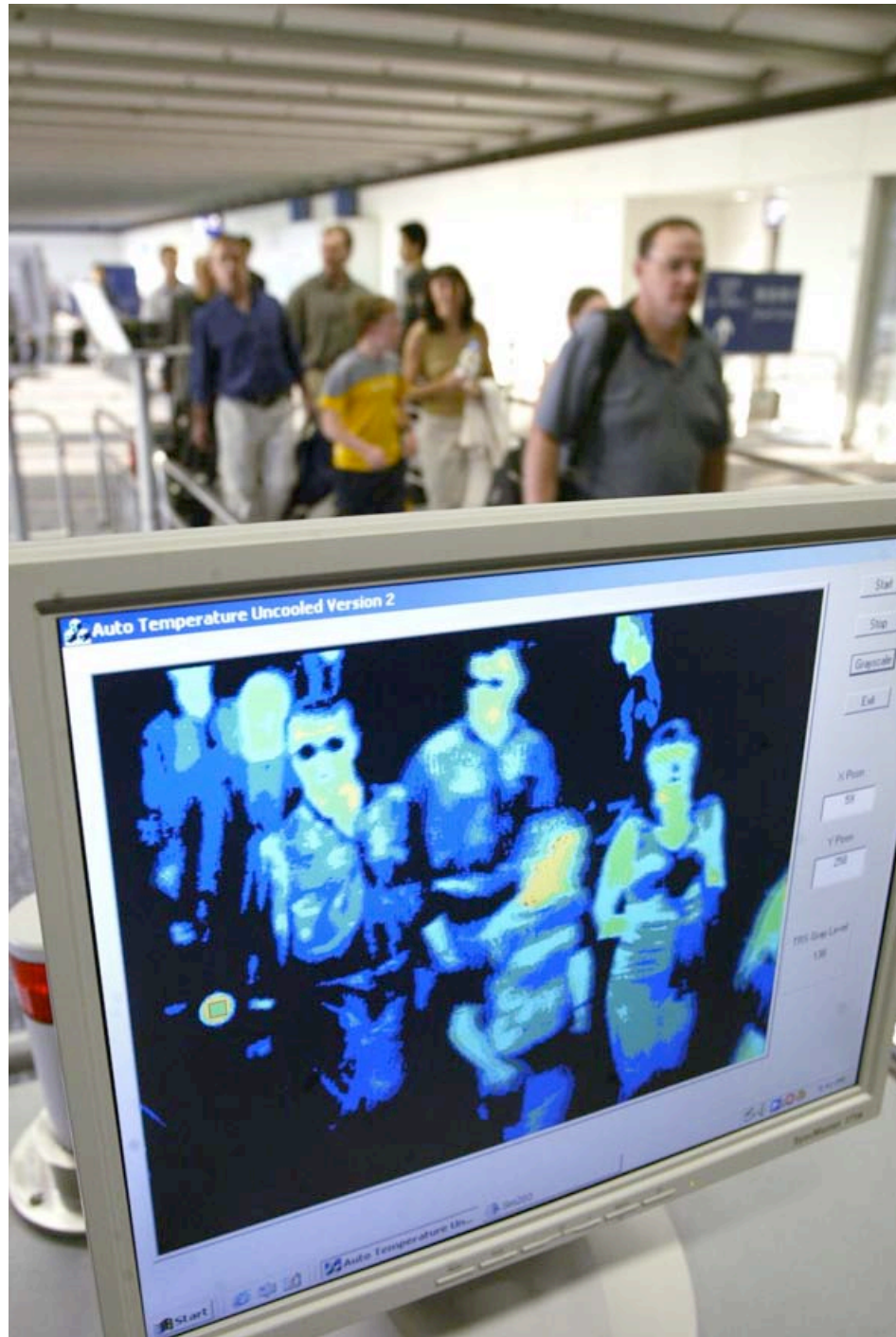
Figure 5: A thermal imaging scanner is used to screen for fevers in incoming passengers inside the arrival hall at Hong Kong International Airport 9 September 2003
