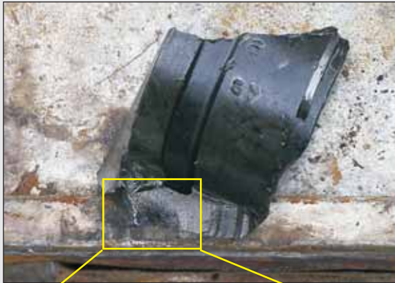
FIGURE 7: Section of piston skirt showing fatigue crack on gudgeon pin socket web section
