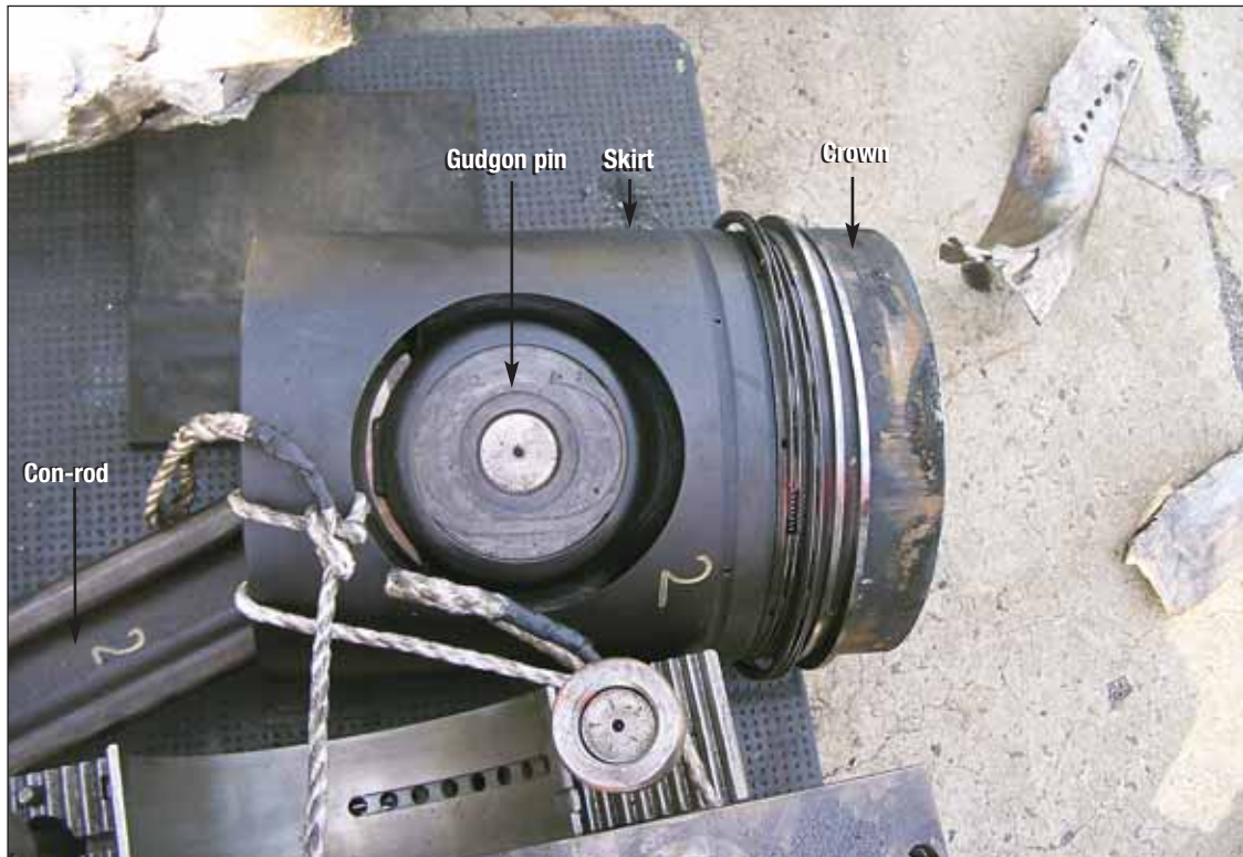
FIGURE 2: Piston assembly on pallet
