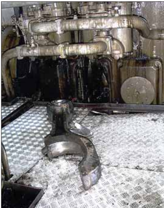
FIGURE 5: Con-rod lying on floor plates as found
