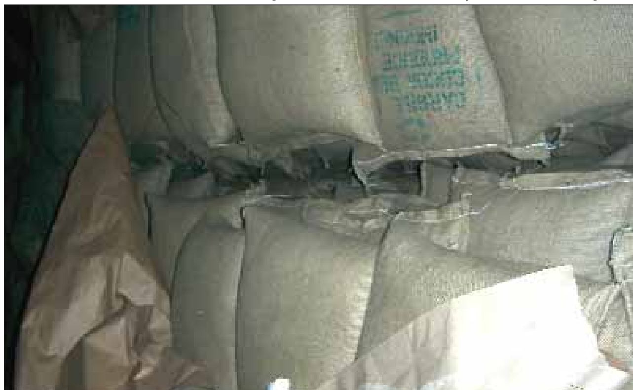
FIGURE 11: Narrow ventilation channel between stacks of cargo in No. 1 hold. Note that some layers are almost touching
