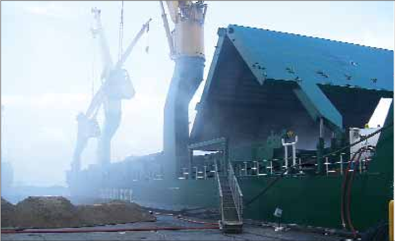
FIGURE 6: No. 2 hold aft hatch panels partially opened
