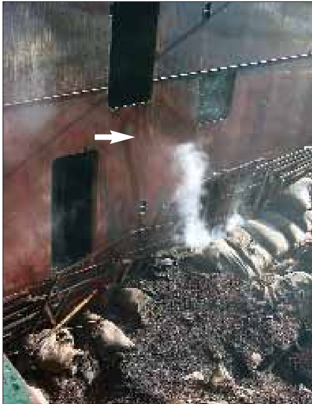
FIGURE 13: Electric cable for cargo light hanging into no.2 hold from hold access
