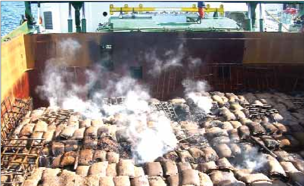
FIGURE 9: Smouldering cargo at aft end of no.2 hold showing burned cavities and channels
