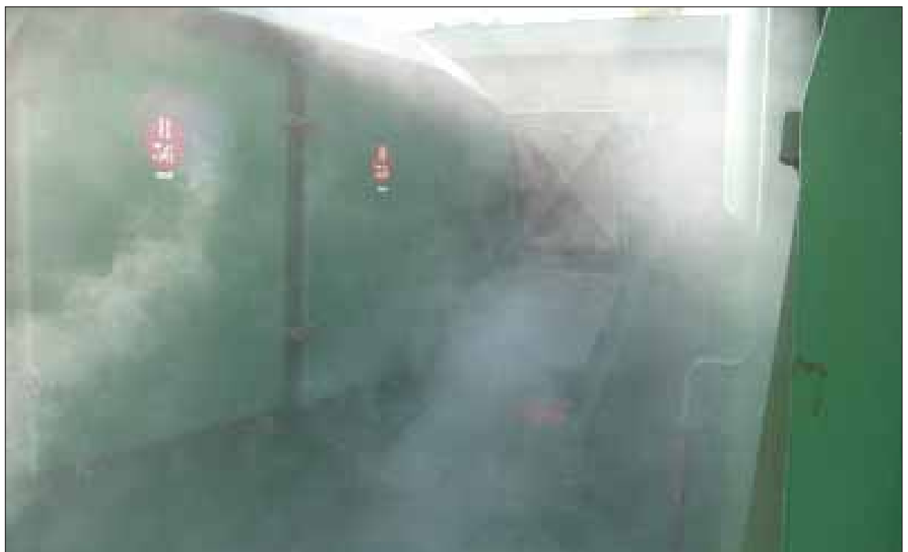
FIGURE 4: Smoke issuing from No. 2 hold access hatch
