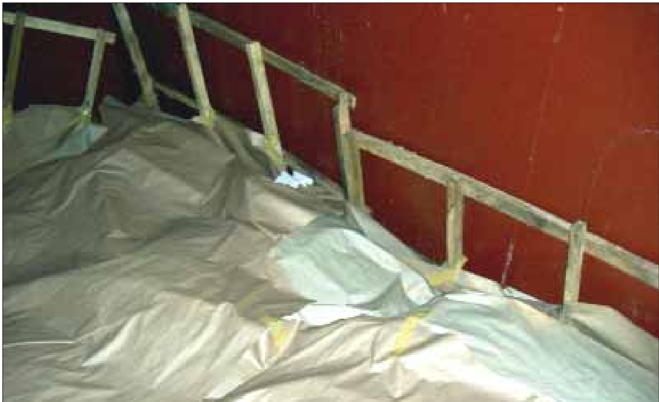
FIGURE 3: Cargo in No. 1 hold, covered with Kraft paper and showing timber dunnage and fumigation sachets of aluminium phosphide
