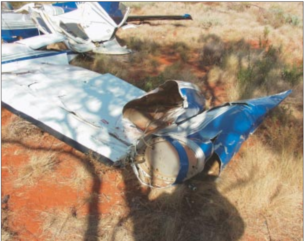
FIGURE 11: Damage to left main fuel tank
