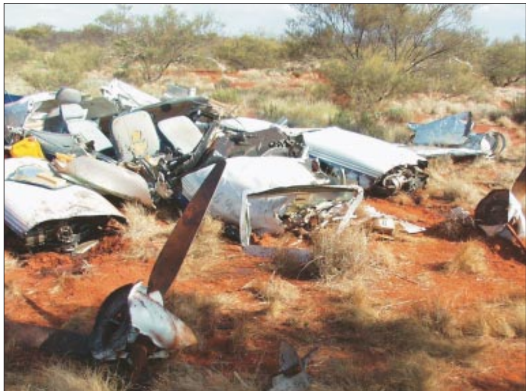
FIGURE 9: View of wreckage from front of aircraft (roof of aircraft cabin cut away by emergency services personnel, prior to arrival of ATSB investigators)
