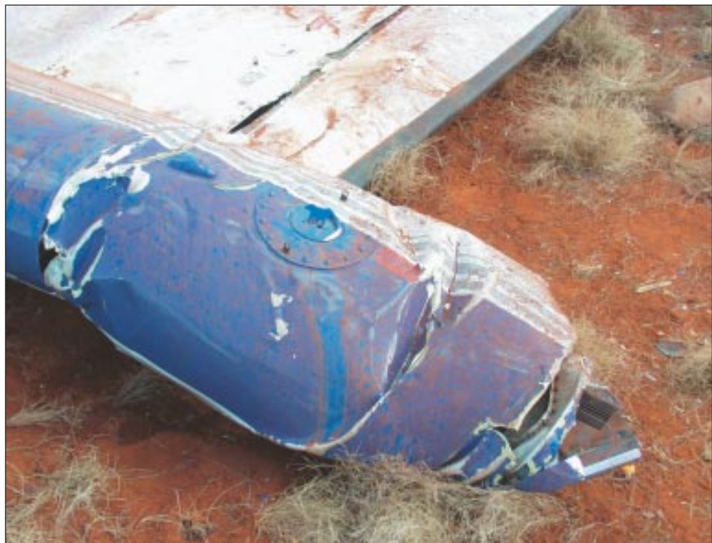
FIGURE 13: Impact damage to right main fuel tank (note fuel cap previously disturbed by emergency services personnel prior to arrival of ATSB investigators)
