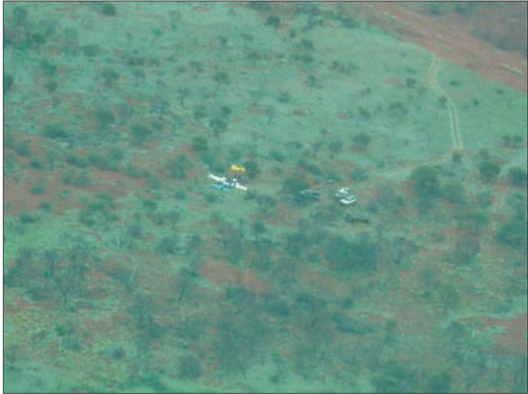
FIGURE 8: Aerial view of aircraft wreckage (note lack of wreckage trail, indicating steep flight path impact angle and low relative forward speed)
