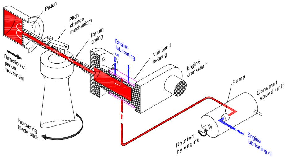
Conversely, when the governor senses that the engine RPM is too low, it allows oil to flow out of the propeller. The spring forces the piston back, which reduces the pitch on the propeller blades and allows the engine to increase RPM (Figure 4).
