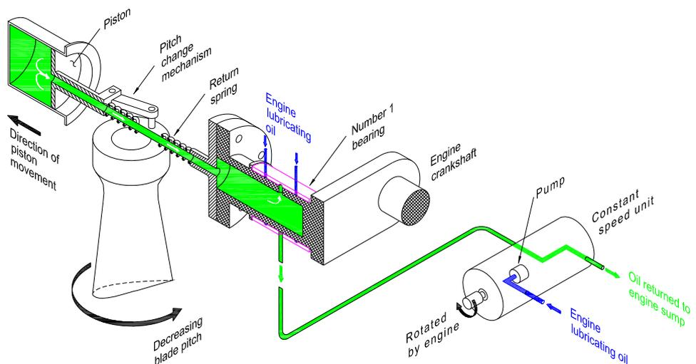
A mechanism in the CSU controls the desired governing speed, allowing the pilot to set the desired engine RPM from the cockpit. During maintenance, the maximum allowable engine RPM is set by adjusting the high speed stop on that control mechanism. To allow for variation in factors, the propeller will normally be capable of moving to a pitch that is less than the maximum governed speed setting when pressure is released from the oil system. This normally only occurs when the engine is shut down.
