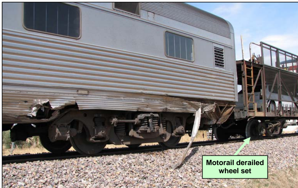
Figure 5: Damage to power van (foreground) derailed bogie of Motorail wagon (background)
