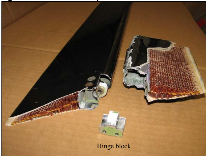
Figure 2: Sections of separated elevator tab
