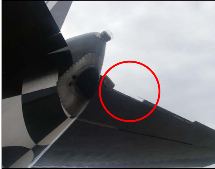
Figure 1: Right elevator tab section detached
