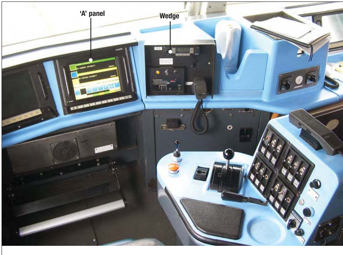
FIGURE 7: Driver's work area showing 'A' panel and wedge radio system
