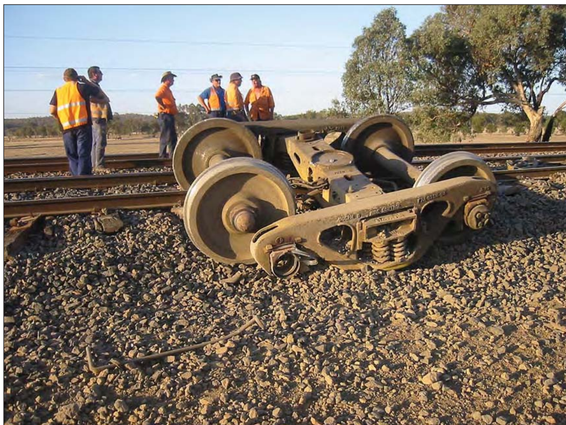
FIGURE 1: Screwed journal within bogie
