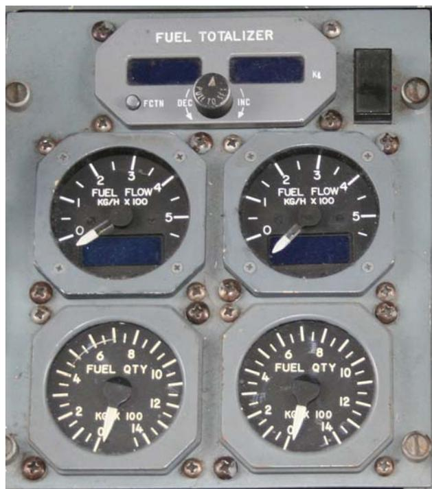
The fuel quantity indicators displayed, in kg x 100, the total fuel quantity in the corresponding wing. The quantity indication was compensated for temperature and fuel density.
