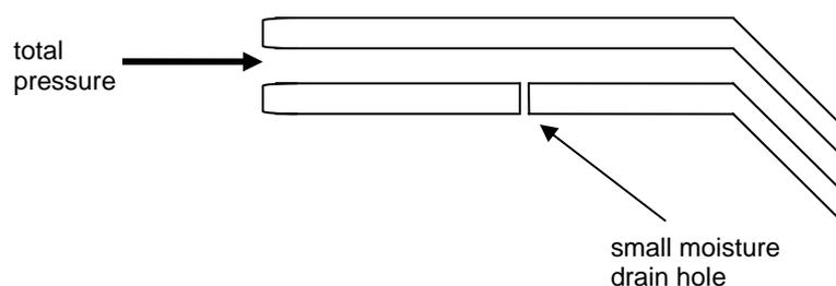
The total pressure measured by the pitot probes was used in the calculation of a number of the flight information variables displayed on the Primary Flight Display.
