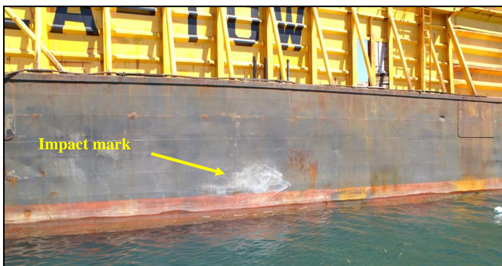
Figure 10: Impact mark on the hull of Seatow 61
