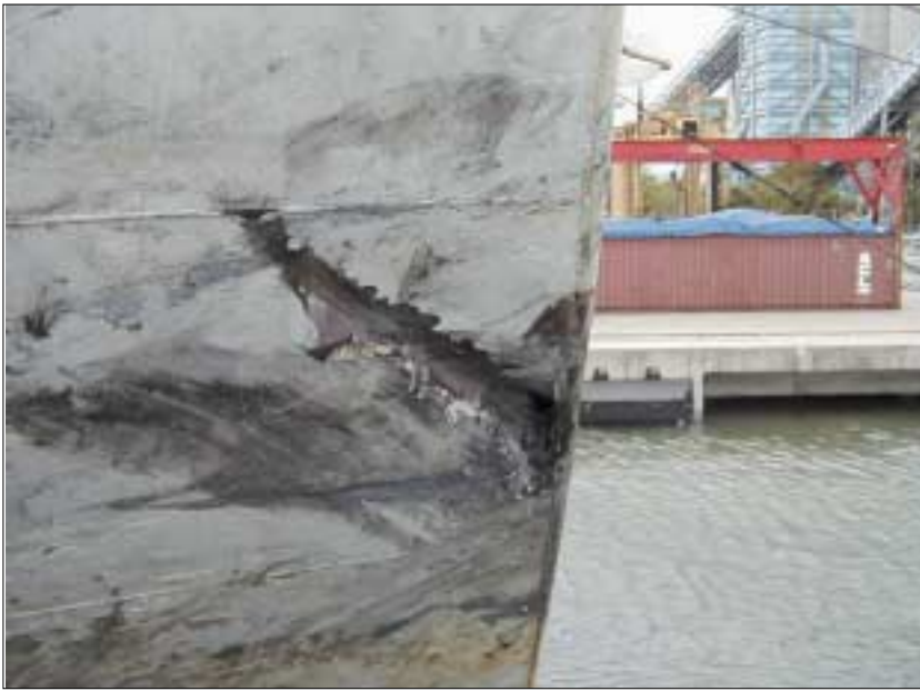
FIGURE 6 Damage to Ariake's hull plating
