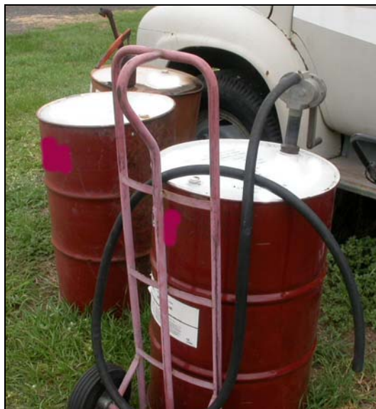
Figure 6: Fuel drum and pump used to fuel the company aircraft the previous night 29
